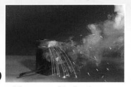
Welding process safely takes place inside the mould.
